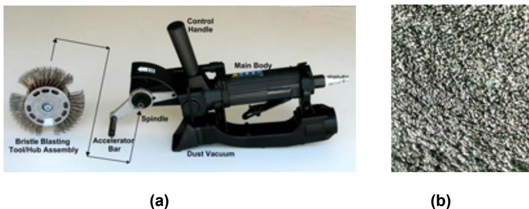
Figure 5 (a) Recently developed bristle blasting power tool system (pneumatic version shown), and (b) characteristic surface generated by bristle blasting process.
